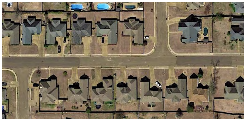
This existing neighborhood in Hernando has many features that prevent it from being a pedestrian-friendly and attractive area. Among those features are a lack of street trees, wide driveways and front parking areas that disrupt the streetscape, and front-loaded garages that project from the house facades toward the street, resulting in a "garagescape" appearance.
